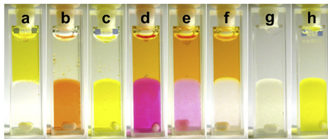
Fig. 16. a) 1- n -butyl-3-methyl-imidazolium hexafluorophosphate, [bmim][PF 6 ] (lower phase), 4',7-dihydroxyflavylium perchlorate in 0.01 M HCl (upper phase), AH + species; b) after moderate shaking, A species; c) after vigorous shaking, AH + species; d) after alkalization of the aqueous phase (pH = 12) with minimum shaking, A - bottom, Ct 2- up; e) after moderate shaking, f) after vigorous shaking, Ct 2- species; g) after reacidification of the aqueous phase and vigorous shaking, Ct species; h) after irradiation of the ionic liquid phase at 366 nm, AH + species [48].
